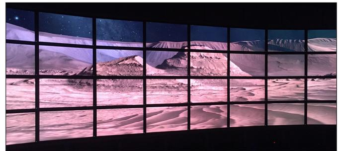
Fig. 6: Browsing the surface of Mars in a clustered environment rendering on the power wall at the University of Utah. The system uses eight rendering nodes, each connected to four screens.
