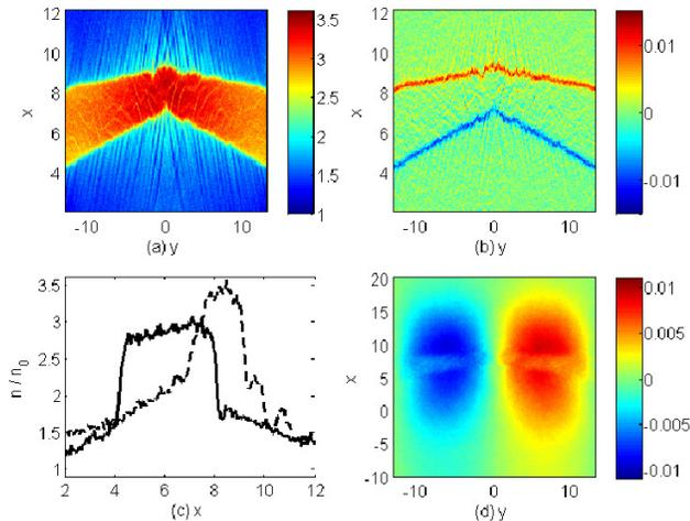
FIG. 5: The ion density distribution expressed in units of  $n_0$  is shown in panel (a). Panel (b) shows the distribution of  $E_x(x,y)$ . The ion density distributions along two slices  $y = 0$  (dashed black) and  $y = 13.1$  (black) are shown in panel (c). Panel (d) shows the distribution of  $B_z(x,y)$ . The time is  $t = 70$ .
