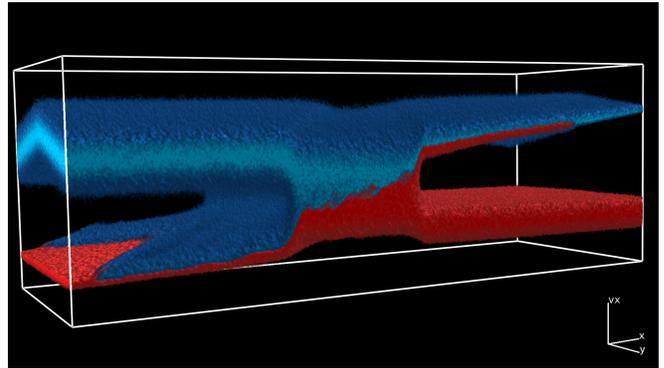
FIG. 6: The ion phase space density distribution  $f_i(x,y,v_x)$  at the time  $t = 70$ . The blast shell ions (blue) are located mainly at high positive values of  $v_x$  while the ambient ions (red) are located mainly at low values of  $v_x$ . The x-axis range is  $[-5.75, 12.0]$ , the y-axis range is  $[-13.1, 13.1]$  and the  $v_x$ -axis range expressed in units of  $c_s$  is  $[-1.9, 5.8]$  (multimedia view).
