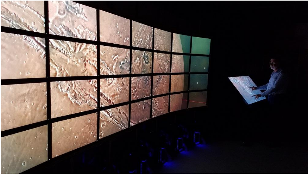
Figure 2. Multi-Touch table driving a power-wall using a linked OpenSpace session such that the viewpoint on the power-wall is controlled by the touch-table. The imagery is the Valles Marineris of Mars obtained from satellites orbiting Mars and streamed to OpenSpace through WMS.
