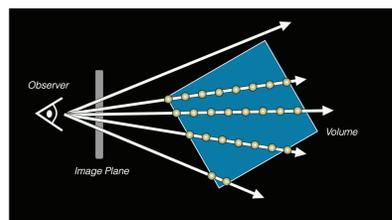
**PIXEL VALUES** For each ray that is cast the pixel value is set by sampling the voxel values along the ray. Transfer functions allow the user to set the opacity and color for each intensity value. Lighting, shading and other rendering settings can be applied for desired image results. IMAGE: LINKÖPING UNIVERSITY
