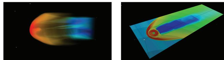
**EARTH'S MAGNETOSPHERE, 20 MAY 2007** Earth's magnetosphere, to the left shown as the full model in which the low pressure tail lobes are clearly visible. In the right image a cut plane has been applied to the same data set. Variable: pressure.
