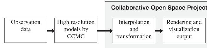
**DATAFLOW** Observation data is used as input for simulations at Community Coordinated Modeling Center (CCMC), resulting in high resolution output models. These are accessed using the Kameleon library developed at CCMC and transformed prior to rendering.
